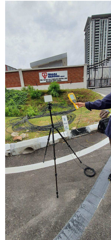
Extremely low frequency electromagnetic field at high voltage cable and substation
